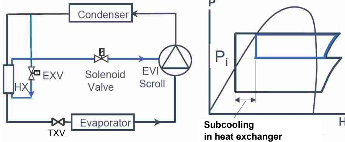
Figure 1-Vapour-injected scroll compressor cycle
