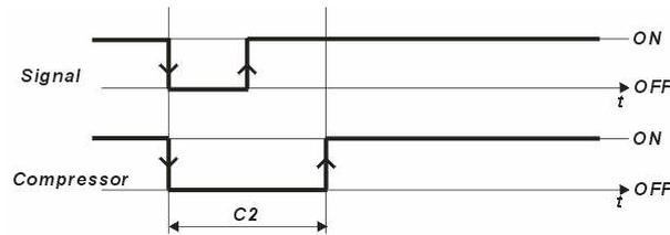
**- Delay between 2 starts of the compressor**
