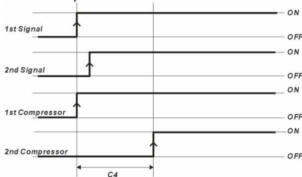
**- Stop delay between compressors**
